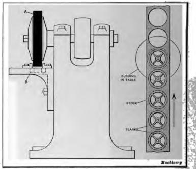
Fig. 14. Machine for Separating Blanks from Stock which has passed through Sub-press Dies
